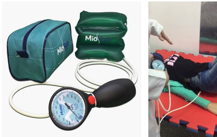
Fig. 1. Pressure assessment equipment. On the left is the MioStab equipment, with its bag and manometer. On the right the equipment in use, under the lumbar region of the volunteer
