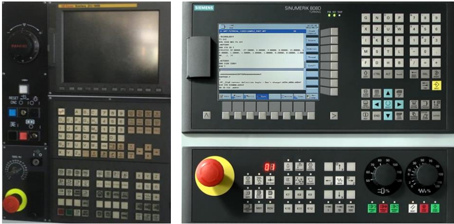
Figure 6. Examples of control panels of CNC machines
