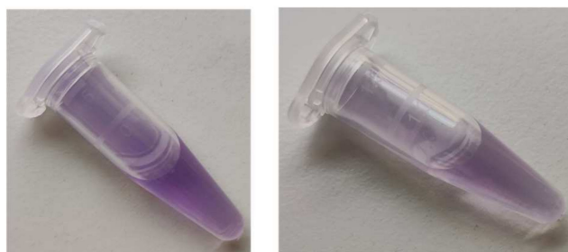
Figure 6. Colors formed by the reaction of BSA (10 mg/mL) with \text{ABTS}^\bullet (107 \mu\text{M} , final concentrations), left, and by the reaction of tyrosine (2 mM) with \text{ABTS}^\bullet (107 \mu\text{M} , final concentrations), right. Reaction volume: 1 mL, reaction time: 1 h.
