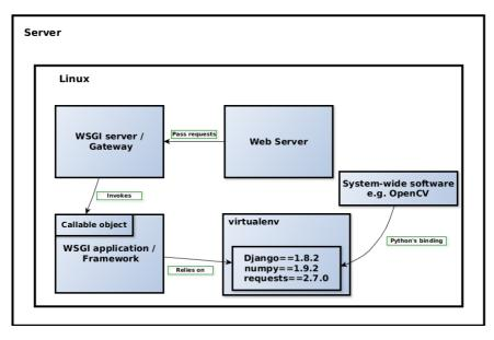
Fig. 1. Configuration of server working with Python (Makai, 2015)
