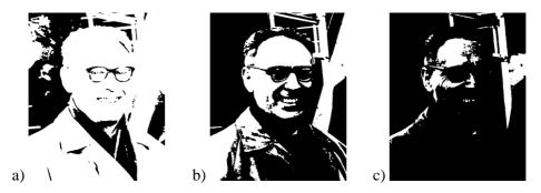
Fig. 3. Simple thresholding with THRESH\_BINARY: a) threshold = 50, b) threshold = 127, c) threshold = 170
