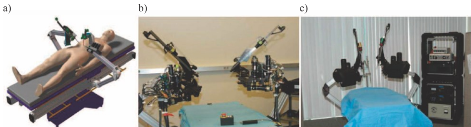
Rys. 16. a) CAD model of the RAVEN system, b) Prototype without covers, c) Complete system with the control box [26]
