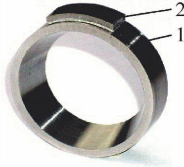
Fig. 1. Friction pair: 1 – ring-shaped sample, 2 – counter sample
