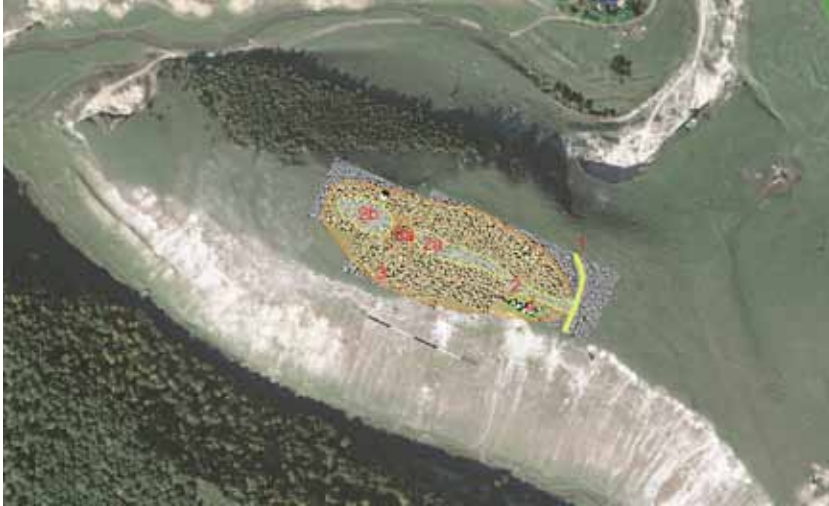
Fig. 7. Gordinești II- Stînca goală , Dist. Edineț. Magnetic map imposed on the satellite image with marked anomalies discussed in the text. 1 – positive linear anomaly caused by the ditch; 2, 2a, 2b – area without dipolar anomalies, interpreted as main communication tract of the settlement and hypothetical internal squares; 3, 3a – area with dipolar anomalies caused by construction clay; 4 – anomalies caused by an archaeological trench
